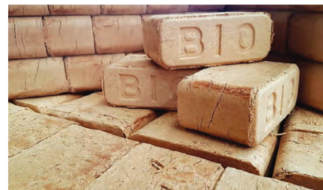
One tonne of BioBriQs is equal to more than four cubic metres of dry firewood, so they take up only about a quarter of the equivalent firewood by energy. They can easily be stored inside, making them easy to access.
